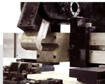
• Booster system for radii till 1D (**) (**) Available optional for all models
